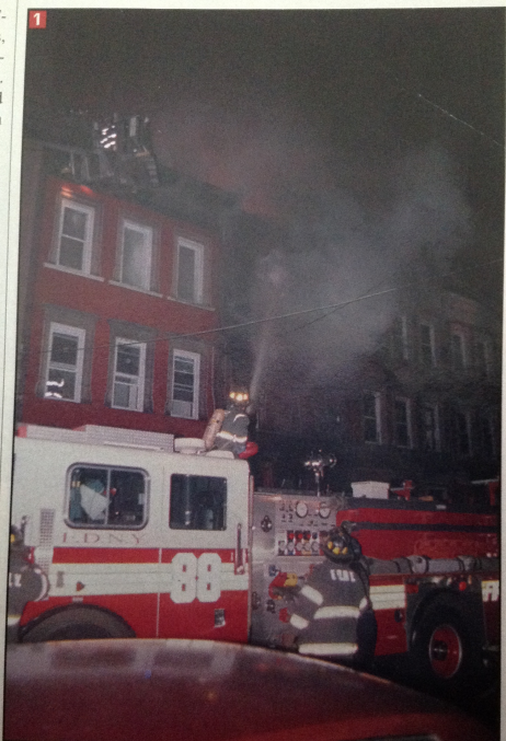
Deck guns are one of the most potent weapons that can be brought to bear at a serious fire. Here a deck gun stream is being used to knock down a heavy body of fire in a vacant building in the Bronx, New York. (Photo by Matthew P. Daly.)
