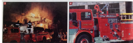
(2) Firefighters are operating a deck gun mounted on the trailer of an aerial ladder at a fire in Boston during the 1970s. Although rare today, the installation of large-caliber stream appliances on aerial ladders (in addition to the ladder pipe nozzle) may prove tactically advantageous. (Photo by Bill Messer.) (3) This tower ladder is equipped with a deck pipe nozzle mounted on the cab roof. The superior positioning options afforded elevating platforms and aerial ladders at serious fires can make the installation of a deck pipe or deck gun nozzle a tremendous asset. (Photo by Peter Alousi.) (4) This engine, which was in service in Schoenectady, New York, in the 1980s, is equipped with a deck gun and a true "deck pipe." The deck gun was supplied directly from the apparatus pump. The deck pipe was supplied by a siamese inlet on each side. With both appliances in operation, more than 2,000 gpm could be applied on a serious fire. (Photo by Andrew A. Fredericks.)
